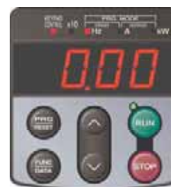
Figure 4.3 Display of the LED Monitor after Power-on
