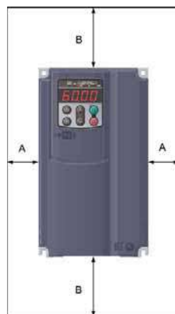
Figure 2.1 Mounting Direction and Required Clearances
